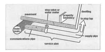
The pipe connecting the mains supply from the water company to your property is called the **service pipe**. The section of the service pipe running from the mains supply to the boundary of your property is the **communication pipe**. The rest of the service pipe from the property boundary into the property is known as the **supply pipe**. The property boundary is usually where the stop valve and water meter are located.
